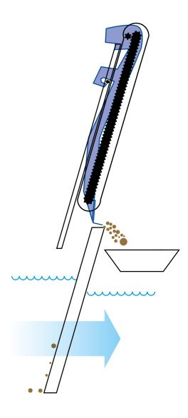
The collected waste is discharged into a container or conveyor
