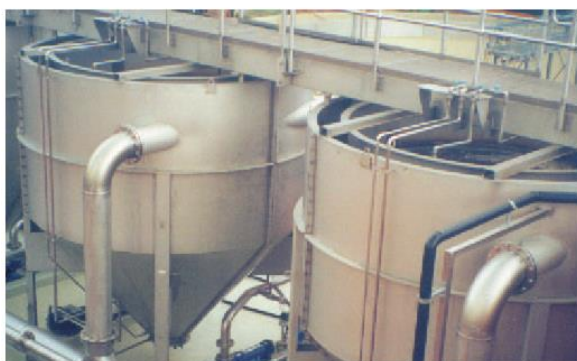
A pair of HUBER Circular Grit Trap HRSF systems
