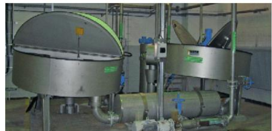
Disc Thickener for volume reduction of process sludge and bio-sludge
