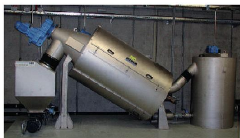
Extremely sturdy: HUBER Rotary Screw Thickener S-DRUM
