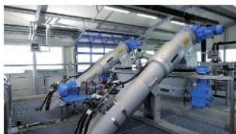
HUBER Membrane Screen ROTAMAT® RoMem Pro especially designed for the removal of hair and fibres
