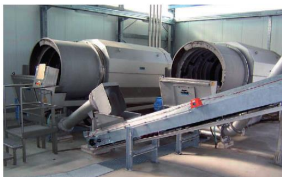
Washing of contaminated grit with the versatile HUBER Wash Drum RoSF9
