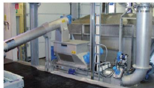
HUBER Wash Press WAP® SL HP: Best screenings washing and compression in a single unit
