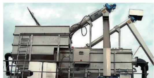
Disc Thickener for volume reduction of process sludge and bio-sludge
