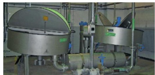
Disc Thickener for volume reduction of process sludge and bio-sludge
