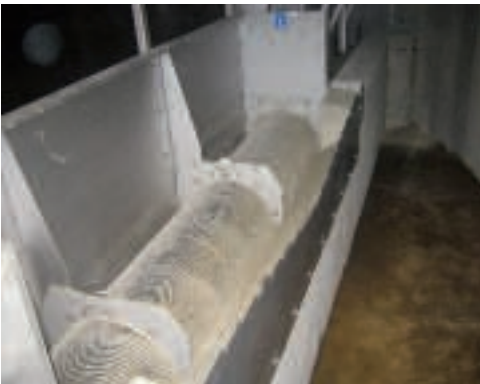
ROTAMAT® Storm Screen RoK 2 combined with discharged flow volume measurement
