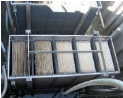
HUBER BioMem® system in container
