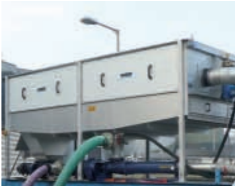
Drum Thickener RoS D for high throughputs
