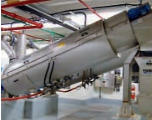
RoS 3 Screw Press Specific power consumption < 0.01 kWh/kg DR
