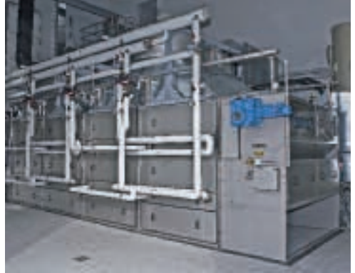
HUBER Belt Dryer BT plus for sludge drying up to > 90 % DS
