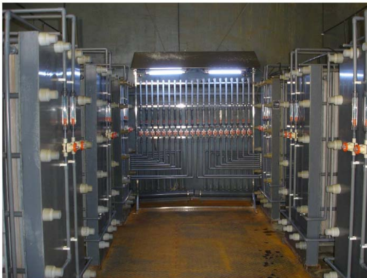
Figure 13. Photograph of a diffusion dialysis unit (installed in 2007, 512 m 2 of membrane area) to recover sulfuric acid from aluminum polishing waste liquor using the new PPO-based anionic membrane (by courtesy of Tianwei Membrane Company).
